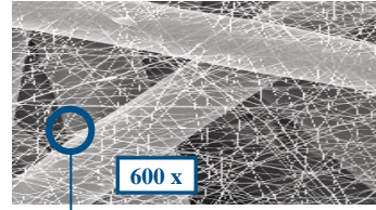
10 Micron Particulate, Ultra-Web ® SB Nanofiber Technology
